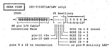
These pins are driven low for 250ms after PWR ON and RESET to allow jumper selectable SCSI ID as shown above.
